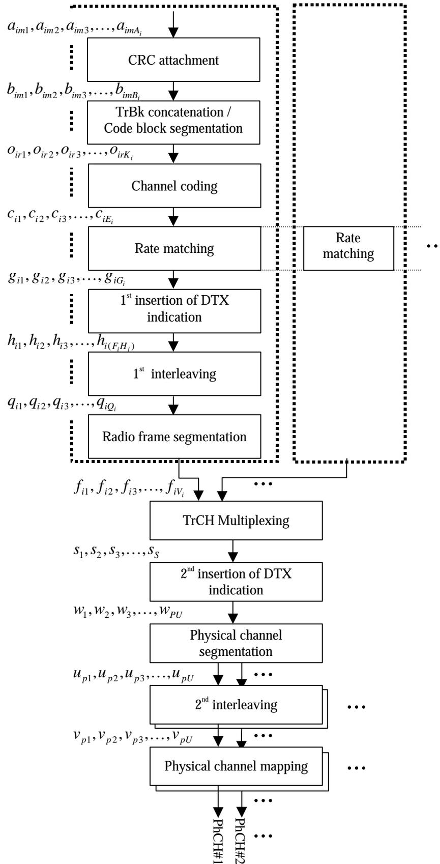
**Figure 2: Transport channel multiplexing structure for downlink**
