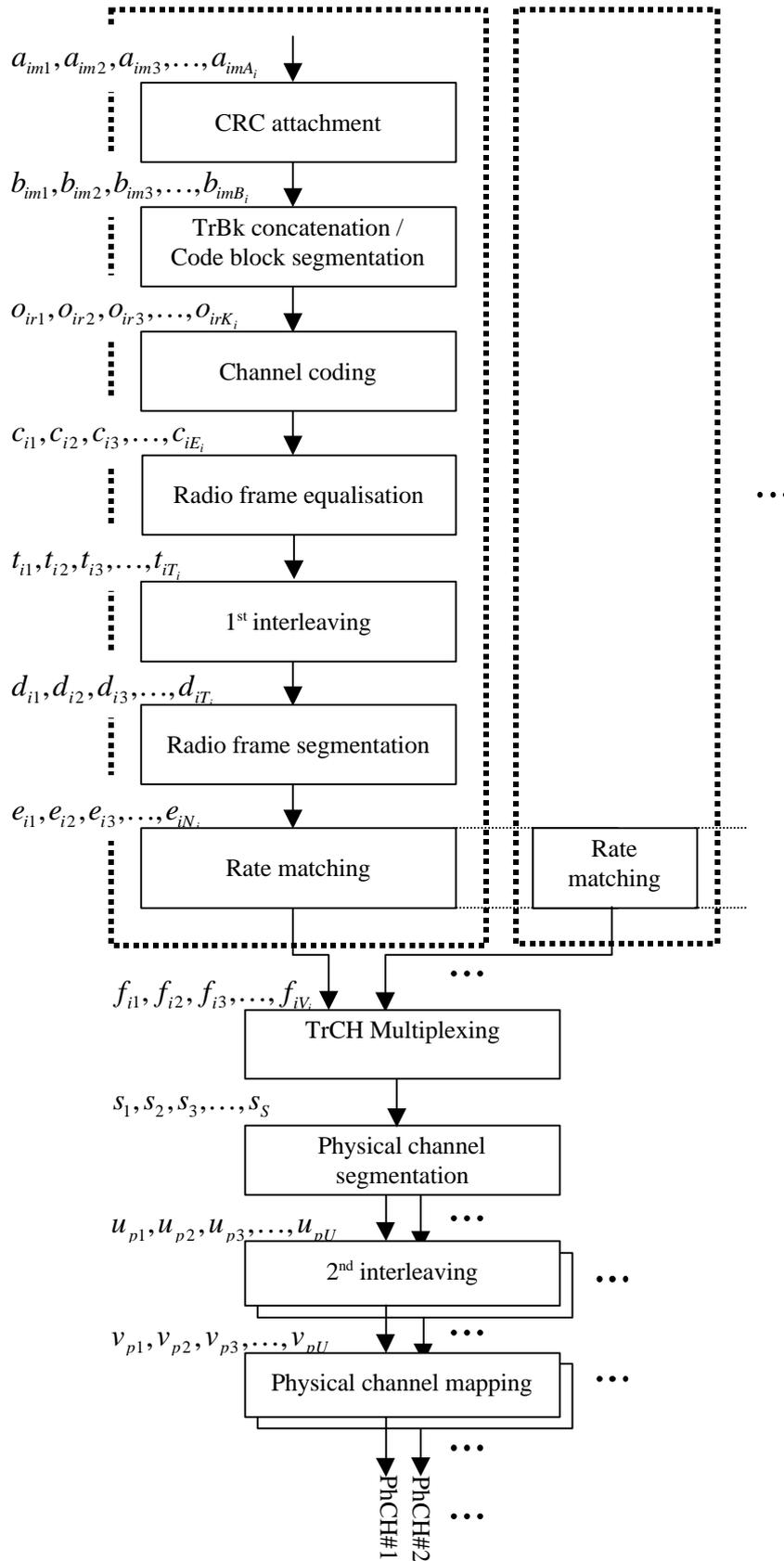
Figure 1: Transport channel multiplexing structure for uplink
