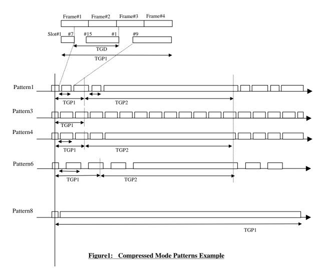
Pattern 1 to 5 uses 7slot TGL. Pattern 6,7 use 14 slots TGL. Using 14 slot TGL may improve cell search time. On the other hand, using 7slot TGL will cause less interference on the system.
