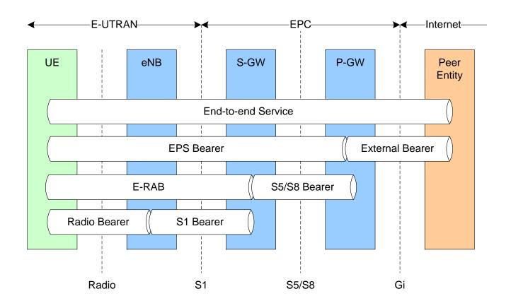
There is a one-to-one mapping EPS Bearer ⇔ E-RAB ⇔ Radio Bearer over the radio interface
