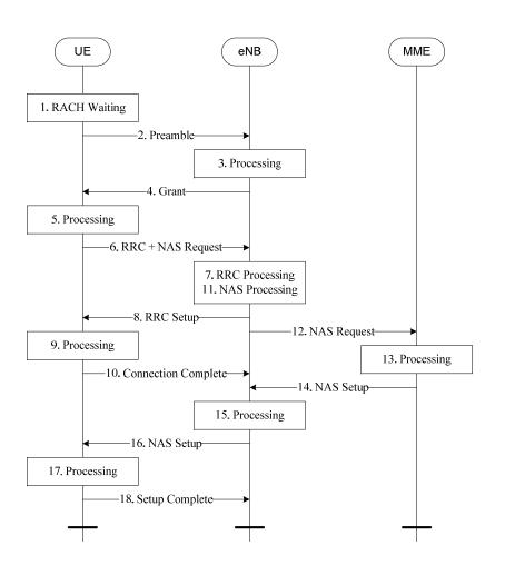
**NOTE:** LTE Rel-8 supports IDLE → CONNECTED latency of around 80ms and, hence, already meets the ITU requirement on C-plane latency for IDLE → CONNECTED transition
