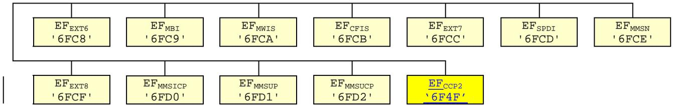
**Figure 4.2: File identifiers and directory structures of USIM**
