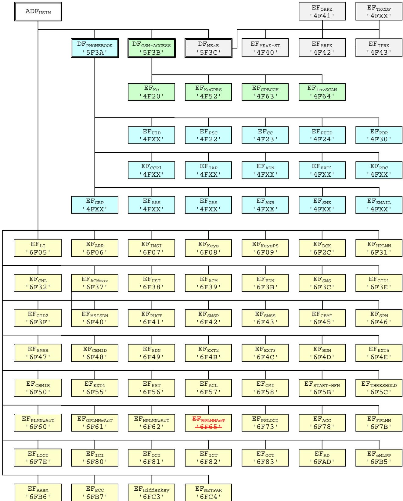
Figure 4.2: File identifiers and directory structures of USIM
