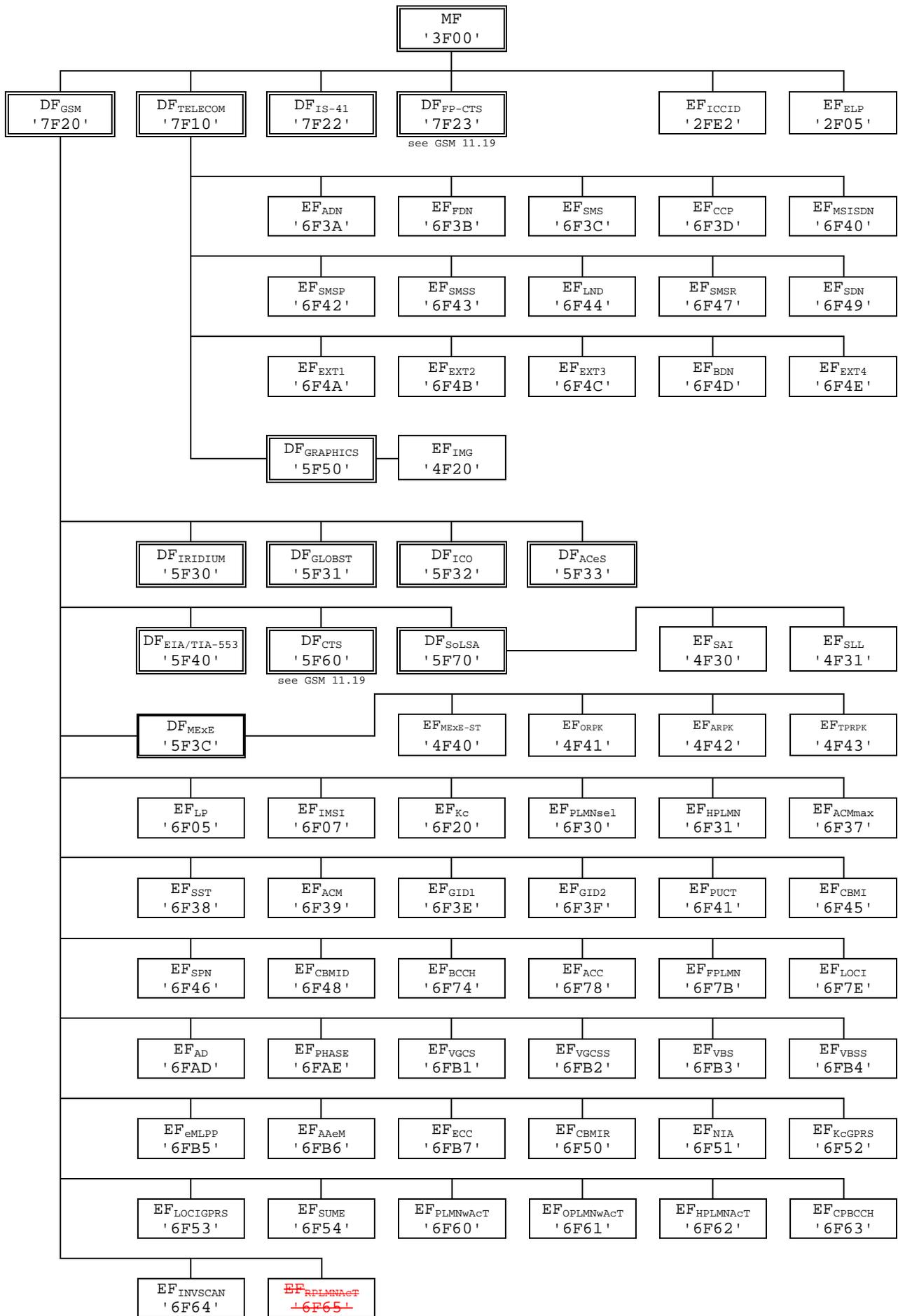
**Figure 8: File identifiers and directory structures of GSM**
