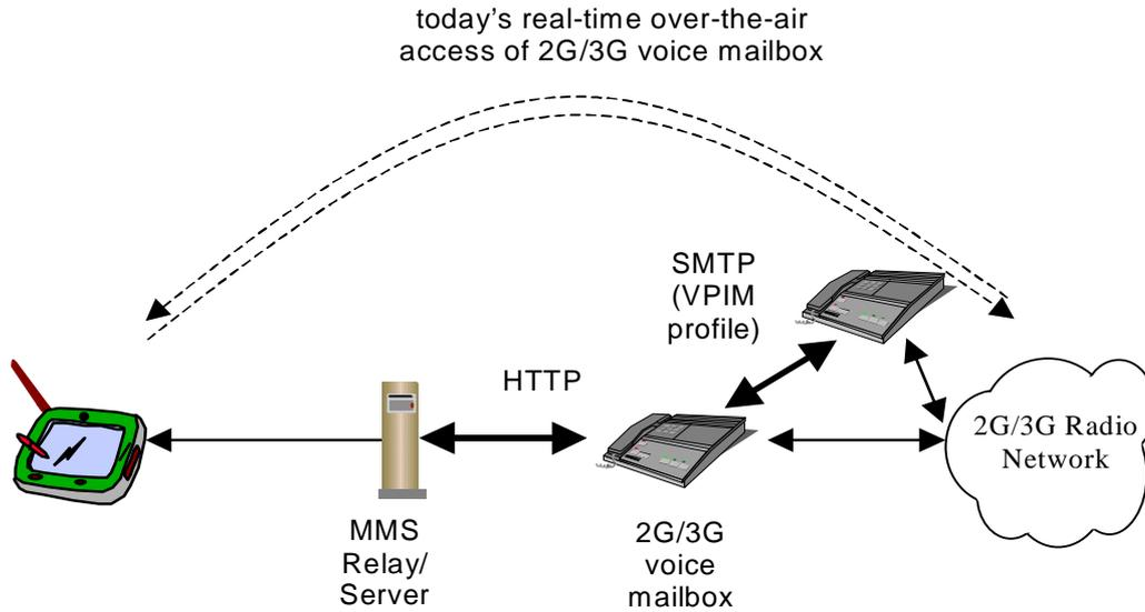
Figure A.5: Second example of MMS interaction with 2G/3G Voice Mailbox based on HTTP
