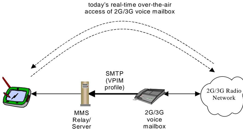
**Figure A.4: First Example of MMS interaction with 2G/3G Voice Mailbox based on VPIM**
