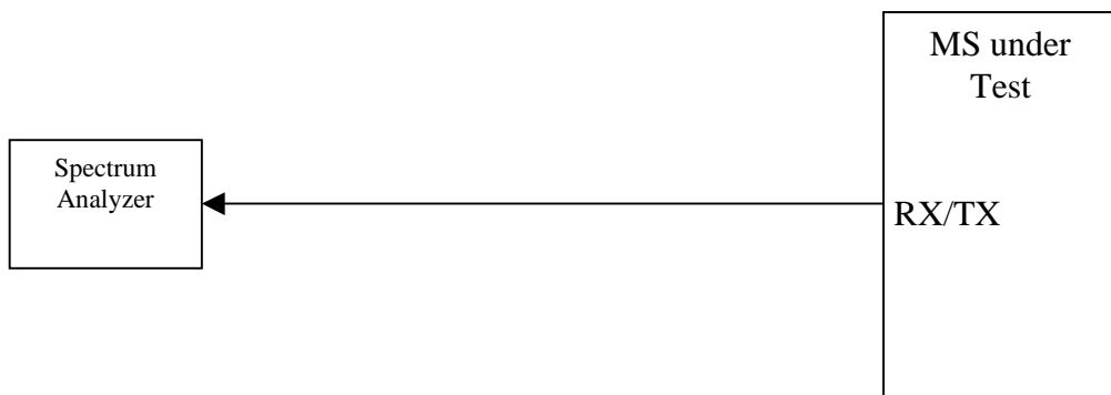
Figure A.8: Connection for Spurious Emission Test
