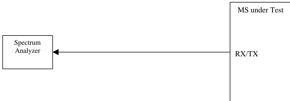
Figure A.8 Connection for Spurious Emission Test
