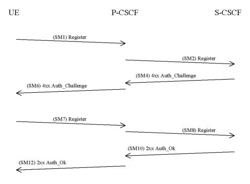
The UE sends a Register message towards the S-CSCF to register the location of the UE and to set-up the security mode, cf. clause 6.1. In order to start the security mode set-up procedure, the UE shall include a *Security-setup*-line in this message.
