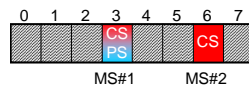
Figure 32 - Example of two GPRS simple class A mobiles; only MS#1 supports single timeslot operation.
