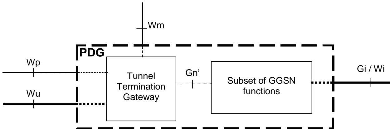
**Figure F.1: PDG implementation re-using GGSN functionality**
