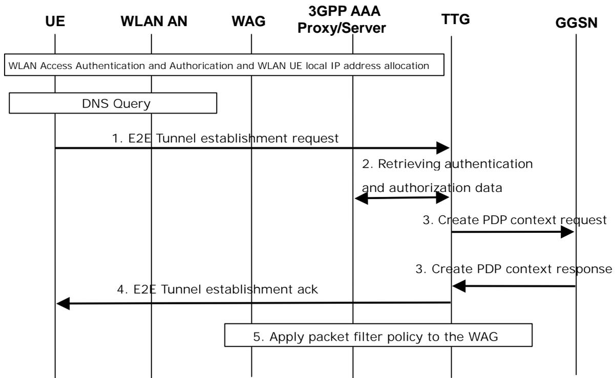
**Figure F.3.1: Tunnel establishment procedure**
