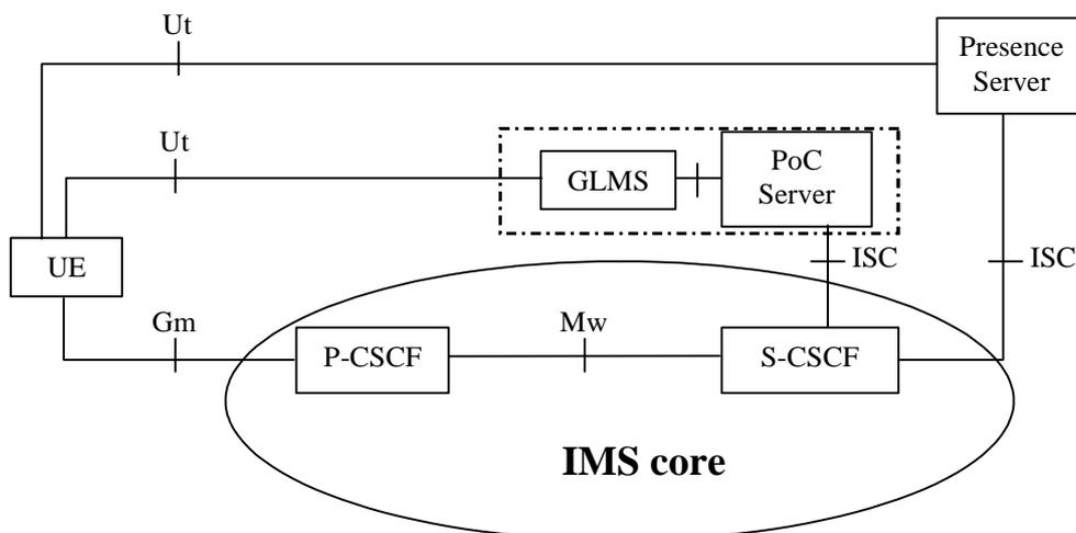
**Figure 5-1. PoC service elements in the IMS architecture**
