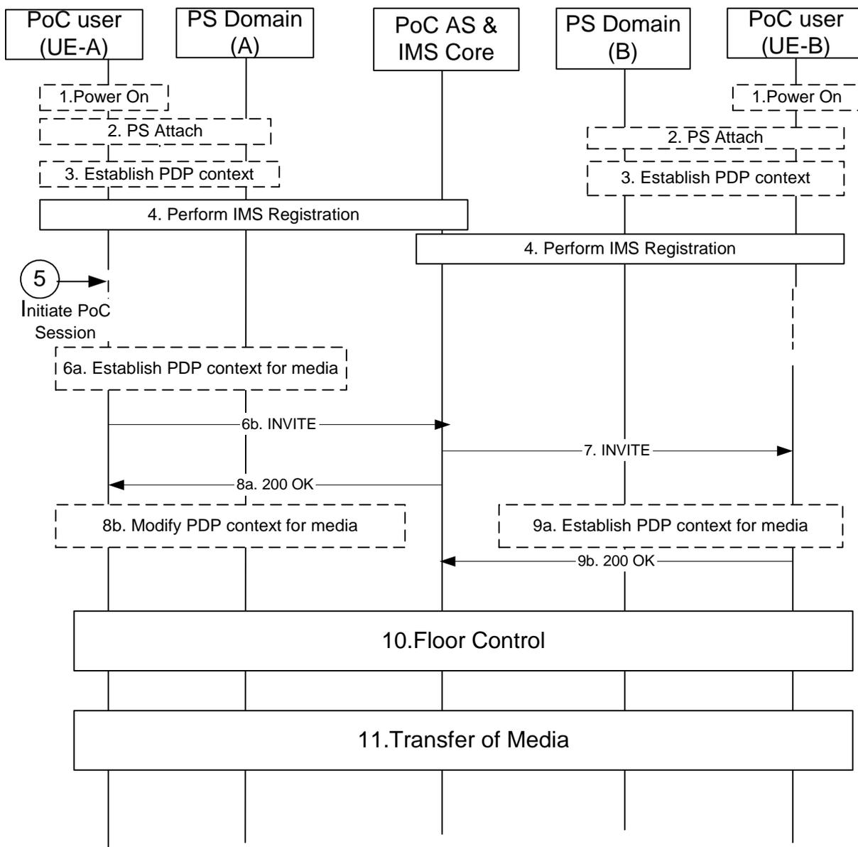
**Figure 5.3.1 Simplified PoC communication based on ‘on demand’ signalling**
