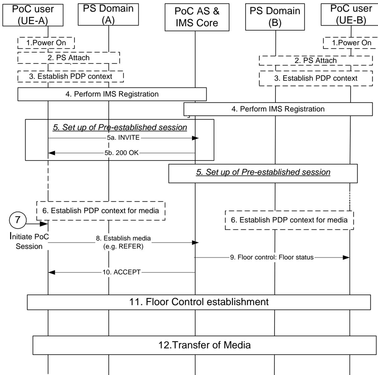
**Figure 5.3.2 Simplified PoC communication based on pre-established session signalling**
