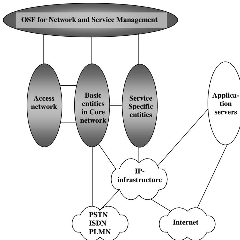
Figure 7.4 : High level **3GPP system UMTS** Network architecture
