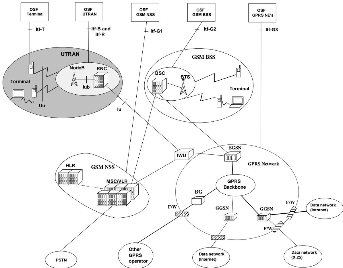
Figure B.1: Overview of a UMTS Network/3GPP System, showing management interfaces and management areas
