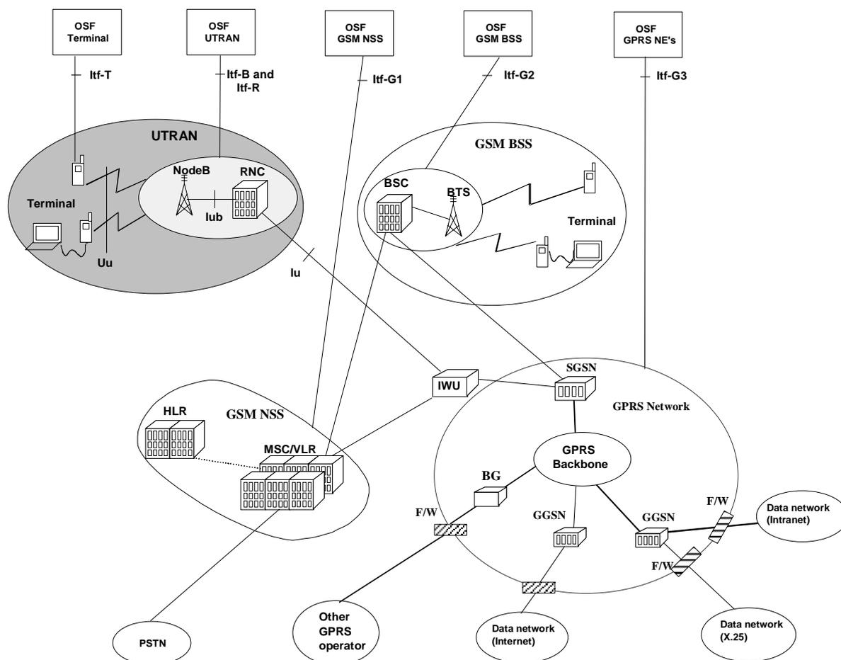
Figure B.1: Overview of a ~~UMTS Network~~3GPP System~~PLMN~~, showing management interfaces and management areas
