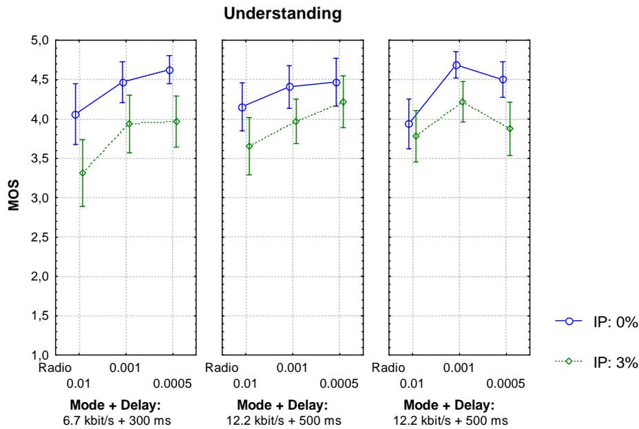
Figure 4: Mean Opinion Scores obtained with the Understanding criterion according to the Radio conditions, the Mode+ Delay, and the IP Packet loss ratio.
