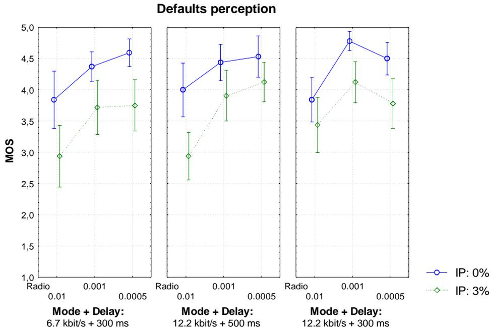
Figure 6: Mean Opinion Scores obtained with the Default perception criterion according to the Radio conditions, the Mode+ Delay, and the IP Packet loss ratio.
