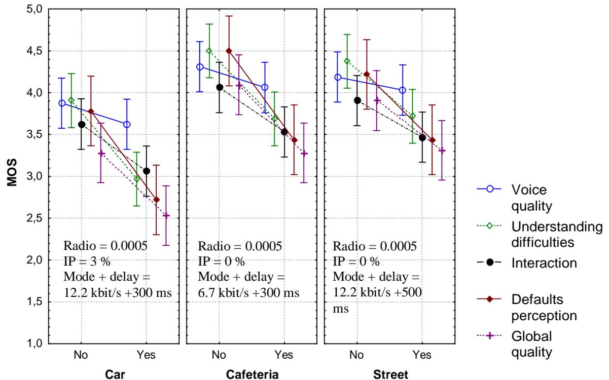
Figure 2: MOS obtained with the five criteria (parameter), according to the type of noise and its presence (Yes/No).
