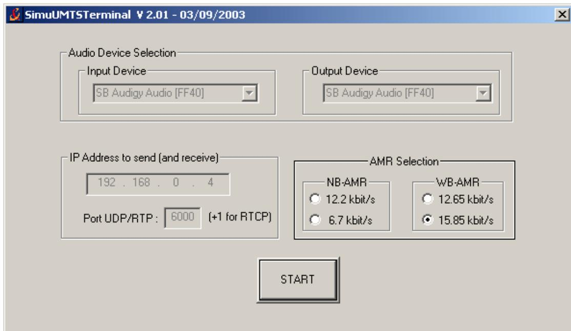
The fields concerning Audio Device selection are filled up automatically. The others fields can be changed but the value in IP Address to send and receive must be 192.168.0.4 as well as the value of the field Port UDP/RTP 6000.
