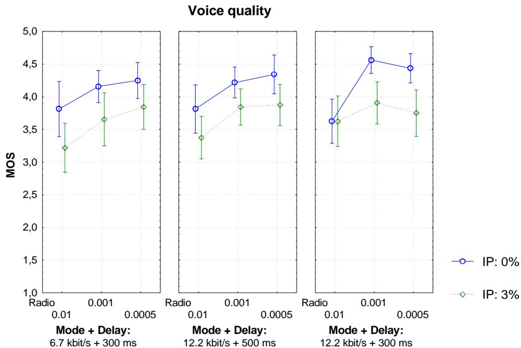
Figure 3: Mean Opinion Scores obtained with the Voice quality criterion according to the Radio conditions, the Mode+ Delay, and the IP Packet loss ratio.
