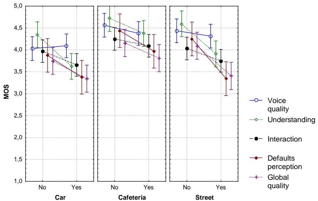
Figure 8: MOS obtained with the five criteria (parameter), according to the type of noise and its presence (Yes/No).
