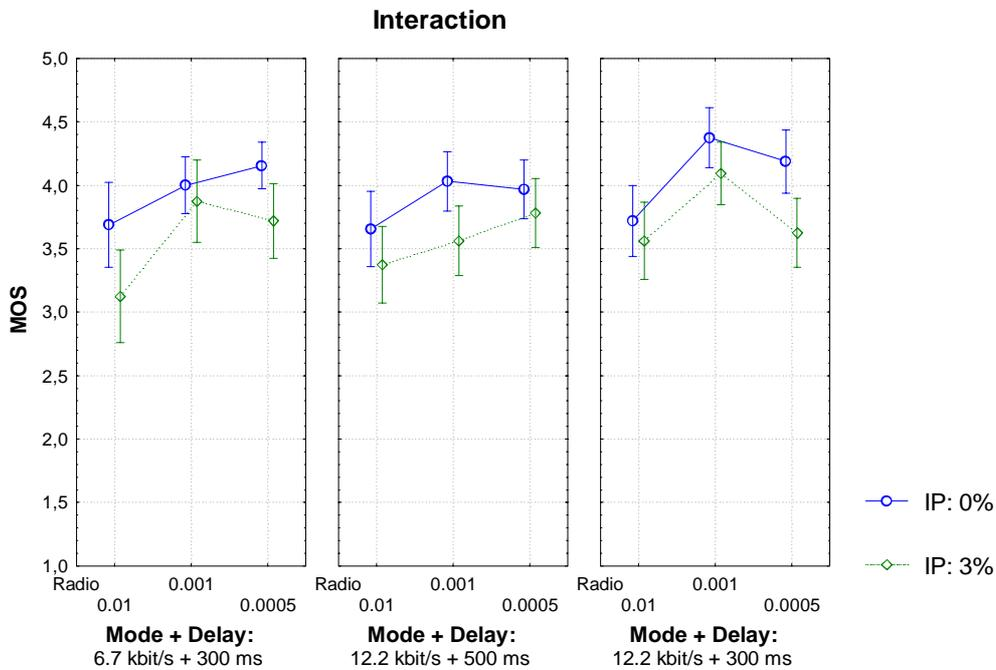
Figure 5: Mean Opinion Scores obtained with the Interaction criterion according to the Radio conditions, the Mode+ Delay, and the IP Packet loss ratio.
