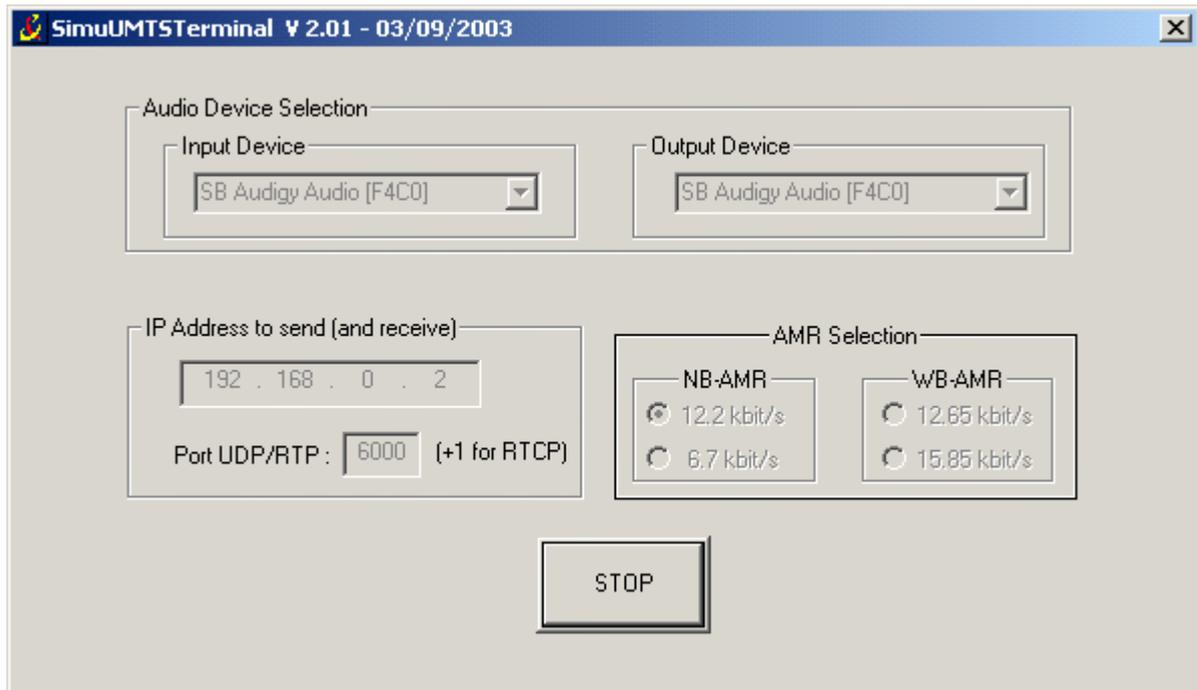
The fields concerning Audio Device selection are filled up automatically. The others fields can be changed but the value in IP Address to send and receive must be 192.168.0.2 as well as the value of the field Port UDP/RTP 6000.
