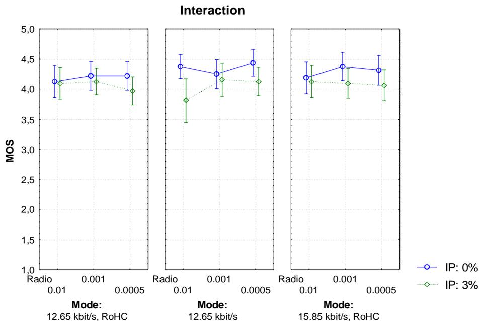
Figure 11: Mean Opinion Scores obtained with the **Interaction** criterion according to the Radio conditions, the Mode+ Delay, and the IP Packet loss ratio.
