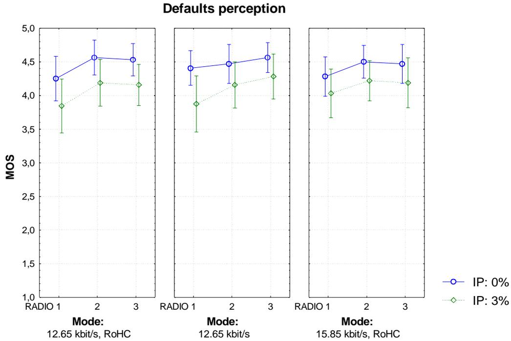
Figure 12: Mean Opinion Scores obtained with the **Defaults perception** criterion according to the Radio conditions, the Mode+ Delay, and the IP Packet loss ratio.
