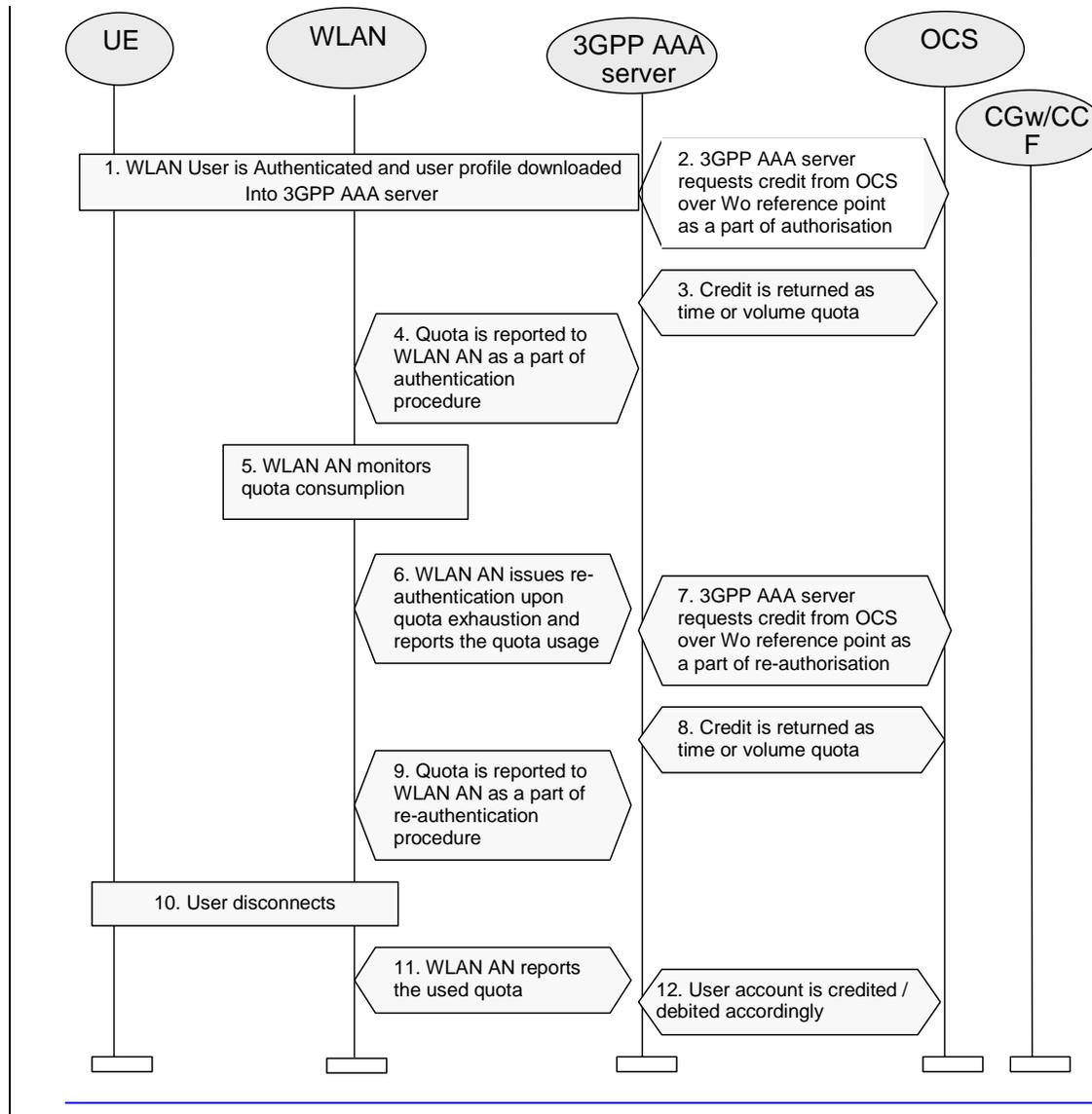
**Figure 7.7 Charging Procedure for Online Charged Subscribers**
