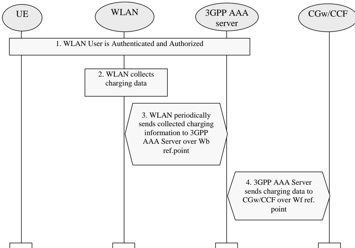
**Figure 7.6 Charging Procedure for Offline Charged Subscribers**
