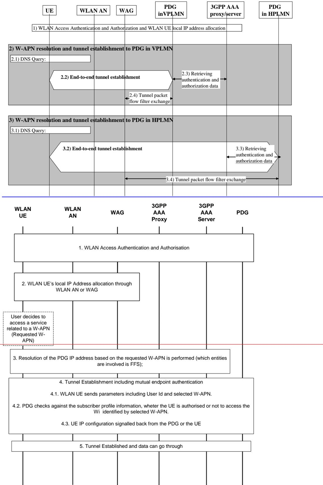
Figure 7.8. Example message flow to WLAN UE-Initiated tunnel establishment
