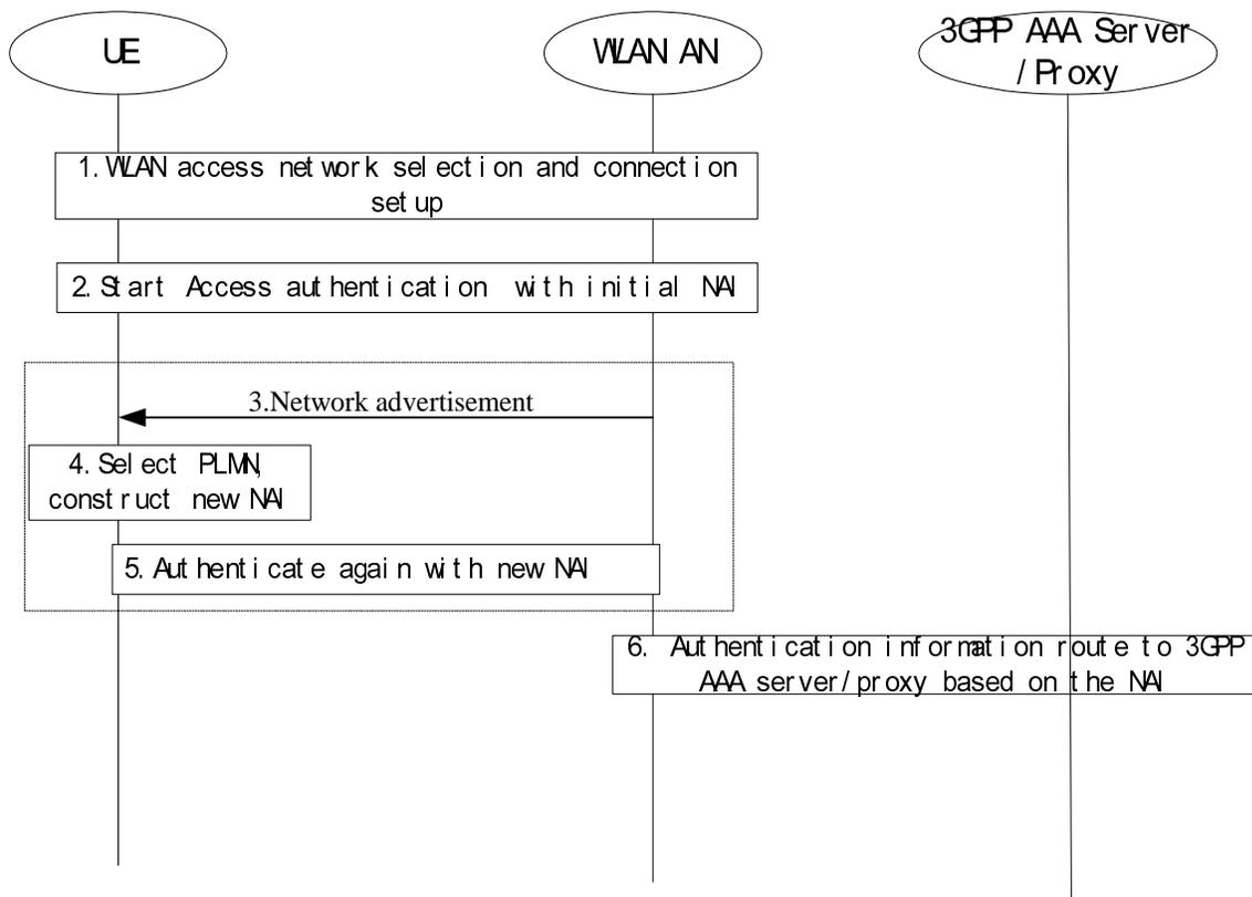
Figure 7.1 WLAN PLMN selection procedure
