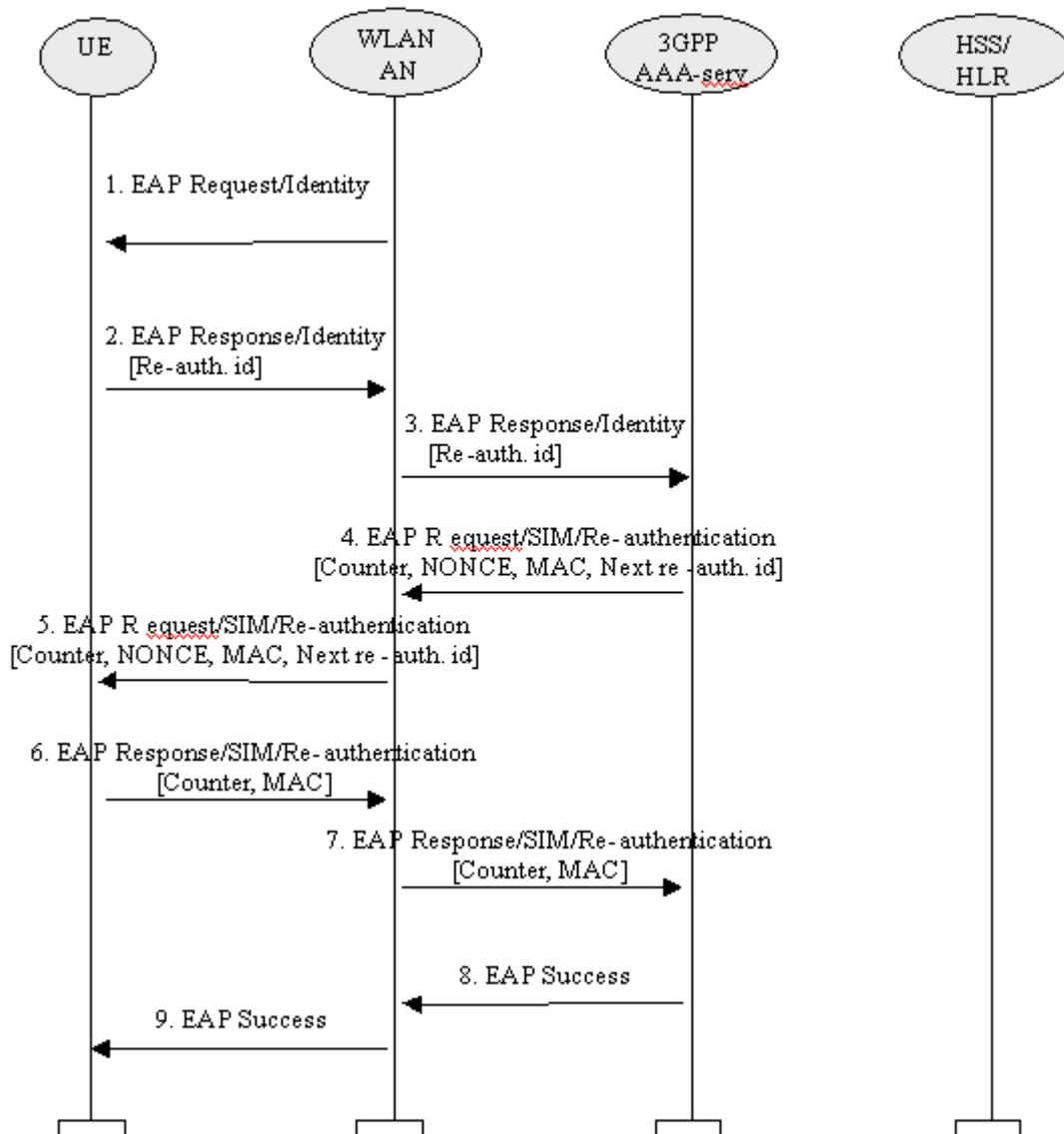
**Figure 7: EAP SIM Re-authentication**
