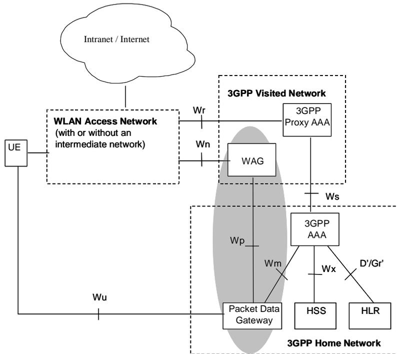
Figure 2: Roaming reference model, services in the HPLMN
