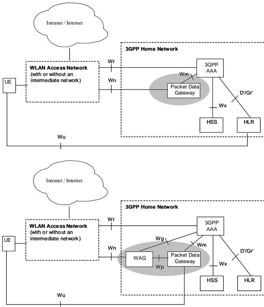
Figure 1: Non roaming reference model
