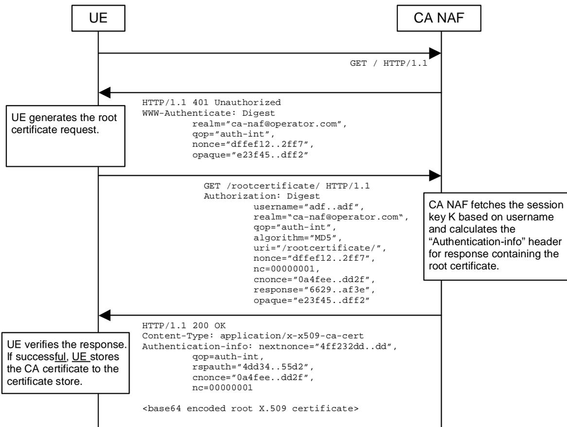
Figure 3: CA certificate delivery with HTTP Digest authentication
