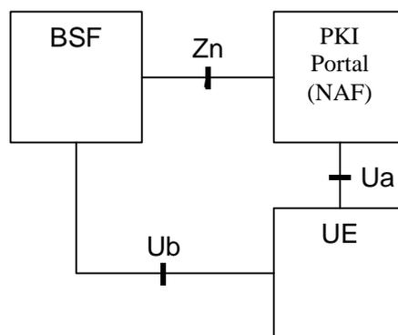
Figure 1: Simple network model for certificate issuing
