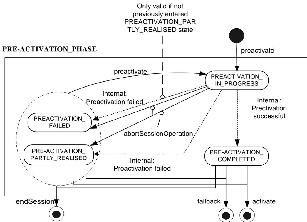
Figure 12: Substate Machine – PREACTIVATION\_PHASE
