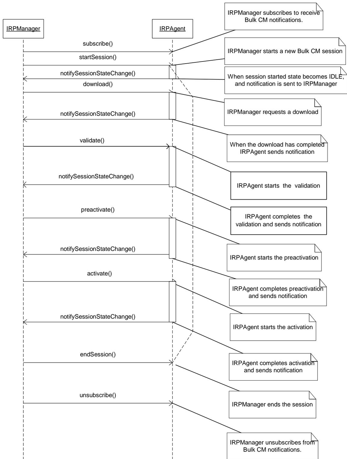
Figure A.3: Example 3: Successful Download and Activation with validation and preactivation.
