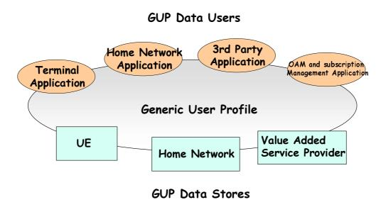
Figure 2: Illustration of the scope of 3GPP Generic User Profile
