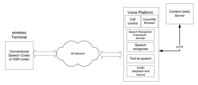
Figure 5 Illustration of the architecture for a typical speech service in a 3G network using network side speech recognition resources based on the speech recognition framework
