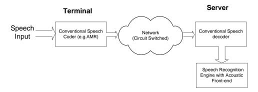
Figure 3 Illustration of Network Based Circuit Switched Speech Recognition
