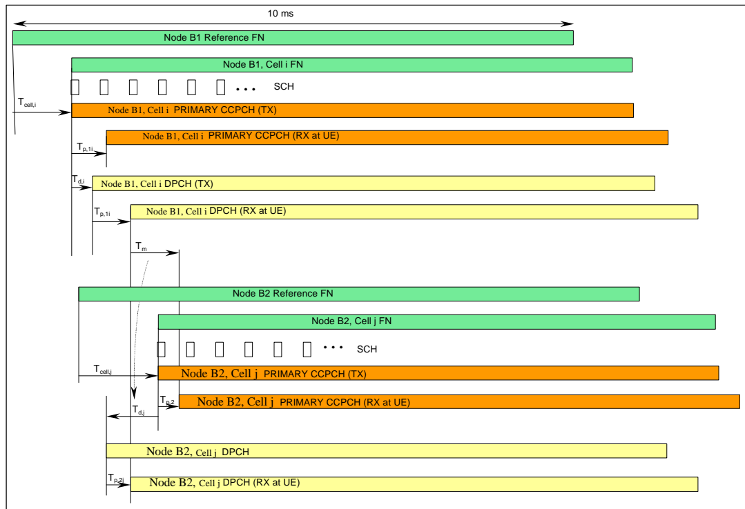
Figure 7. Physical channel timing parameters
