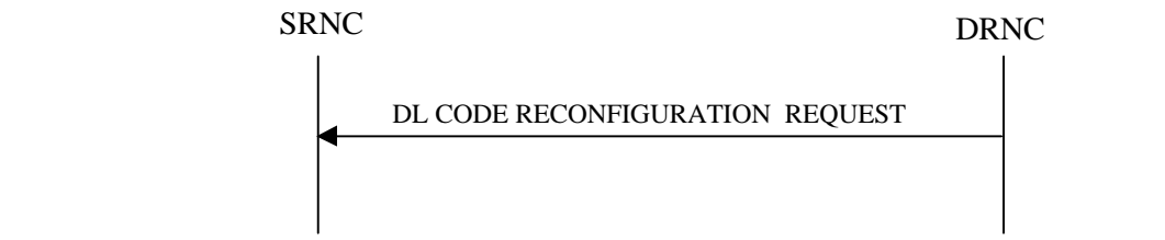
Figure 9-7. An example RNSAP message flow at I_{ur} interface for DL Code Reconfiguration trigger
