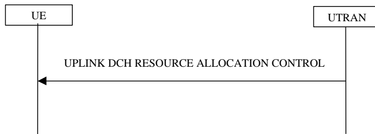
Figure 1: Dynamic Resource Allocation Control of Uplink DCH
