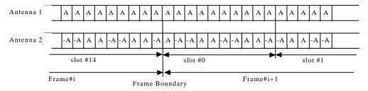
This shows the pattern of two antenna TxD pilot symbol transmission where A = 1 + j.
