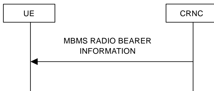
Figure 8.3.3: MBMS radio bearer information signalling flow
