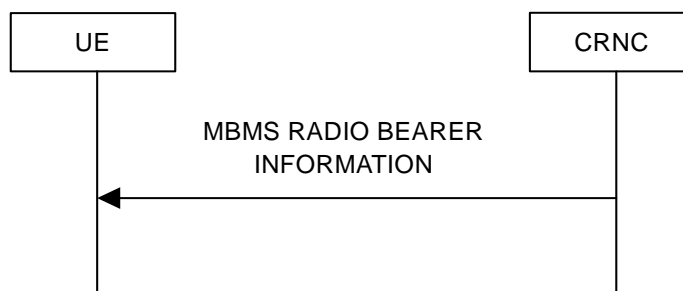
Figure 8.3.3: MBMS radio bearer information signalling flow
