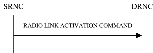
Figure 26D: Radio Link Activation procedure
