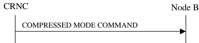
Figure 47: Compressed Mode Command procedure, Successful Operation
