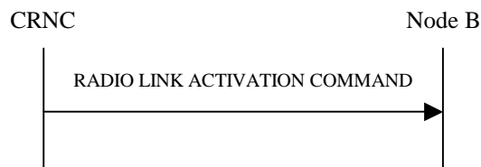
Figure 47D: Radio Link Activation procedure
