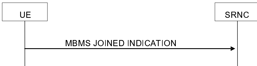
Figure 36: MBMS joined indication signalling flow
