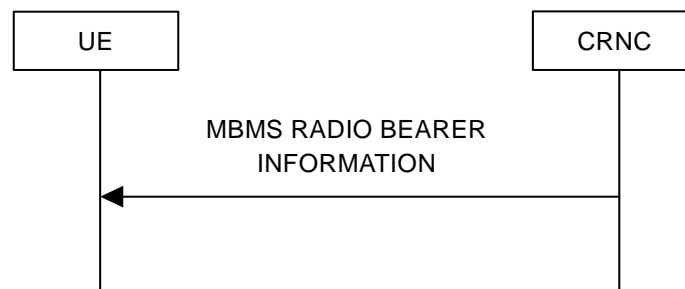
Figure 33: MBMS radio bearer information signalling flow
