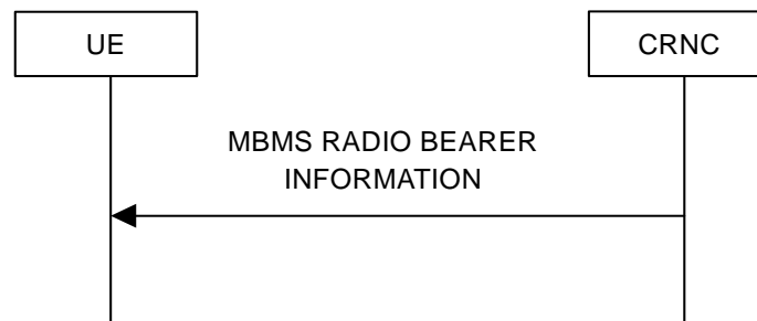
Figure 33: MBMS radio bearer information signalling flow
