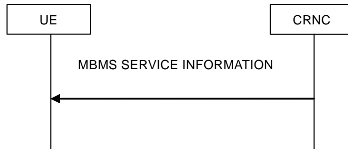
Figure 32: MBMS service information signalling flow
