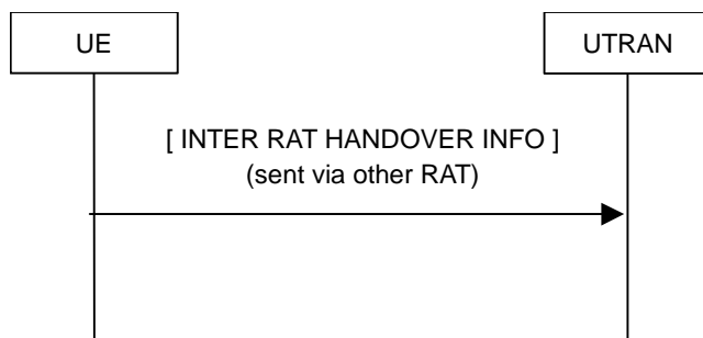
Figure 8.1.16-1: Inter RAT handover information transfer, normal flow
