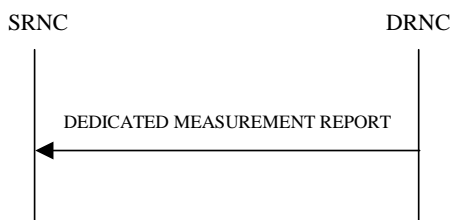
Figure 22: Dedicated Measurement Reporting procedure, Successful Operation
