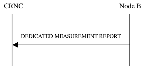
Figure 40: Dedicated Measurement Reporting procedure, Successful Operation
