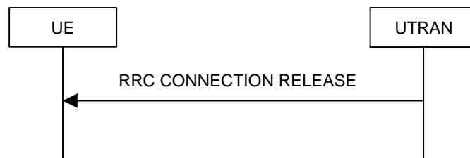
Figure 8.1.4-2: RRC Connection Release procedure on the CCCH
