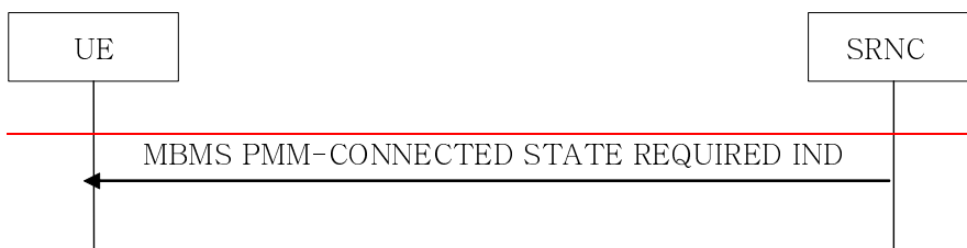
Figure 27: MBMS PMM-CONNECTED state required indication signalling flow
