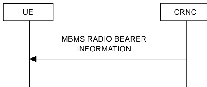
Figure 33: MBMS radio bearer information signalling flow
