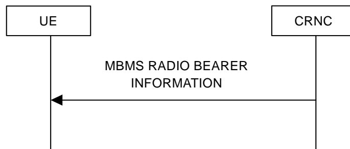
Figure 36363225 : MBMS radio bearer information signalling flow
