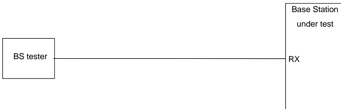
Figure B.15a: Functional Set-up for Verification of the internal BLER calculation for BS without Rx diversity
