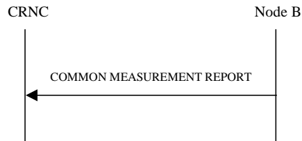
Figure 13: Common Measurement Reporting procedure, Successful Operation
