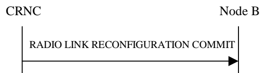
Figure 32: Synchronised Radio Link Reconfiguration Commit procedure, Successful Operation
