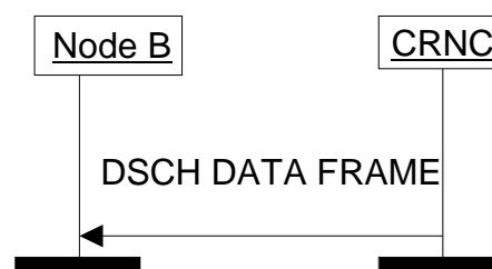
Figure 5: DSCH Data Transfer procedure
