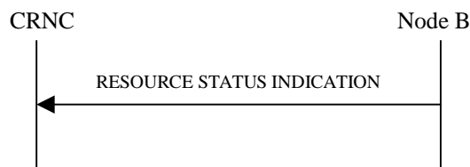
Figure 21: Resource Status Indication procedure, Successful Operation
