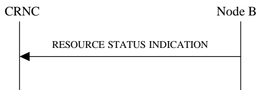
Figure 21: Resource Status Indication procedure, Successful Operation
