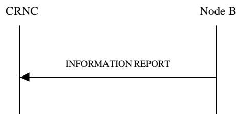
Figure 27N: Information Reporting procedure, Successful Operation
