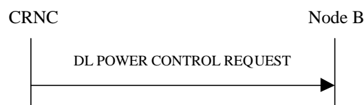
Figure 37: Downlink Power Control procedure, Successful Operation
