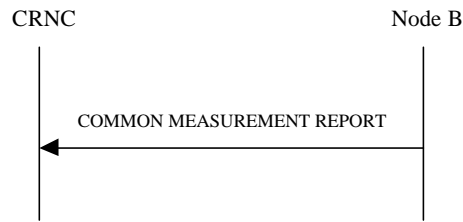
Figure 13: Common Measurement Reporting procedure, Successful Operation
