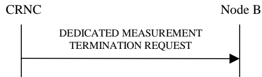
Figure 41: Dedicated Measurement Termination procedure, Successful Operation
