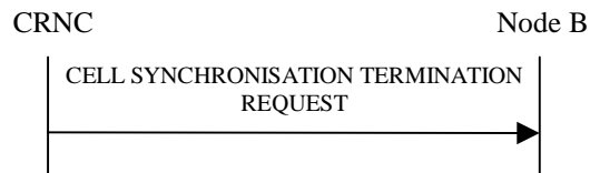
Figure 27H Cell Synchronisation Termination procedure, Successful Operation
