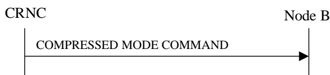
Figure 47: Compressed Mode Command procedure, Successful Operation
