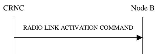
Figure 47D: Radio Link Activation procedure
