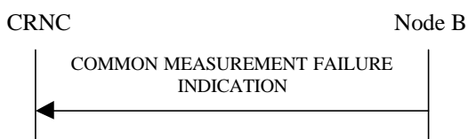
Figure 15: Common Measurement Failure procedure, Successful Operation
