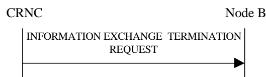
Figure 27O: Information Exchange Termination procedure, Successful Operation
