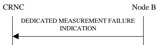
Figure 42: Dedicated Measurement Failure procedure, Successful Operation
