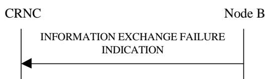
Figure 27P: Information Exchange Failure procedure, Successful Operation
