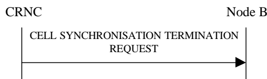
Figure 27H Cell Synchronisation Termination procedure, Successful Operation
