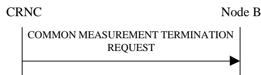
Figure 14: Common Measurement Termination procedure, Successful Operation
