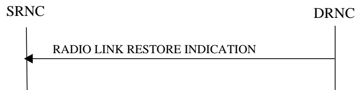
Figure 19: Radio Link Restoration procedure, Successful Operation
