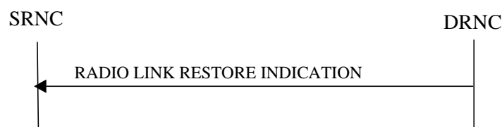
Figure 19: Radio Link Restoration procedure, Successful Operation
