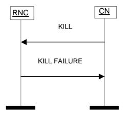
Figure 4: Kill Procedure: Un-Successful Operation
