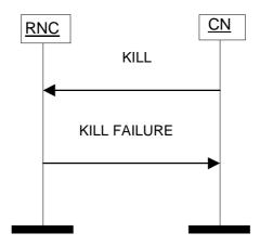
Figure 4: Kill Procedure: Un-Successful Operation
