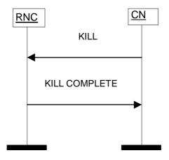
Figure 3: Kill Procedure: Successful Operation
