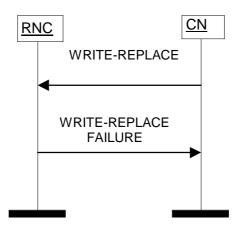
Figure 2: Write-Replace Procedure: Un-Successful Operation
