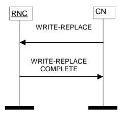
Figure 1: Write-Replace Procedure: Successful Operation
