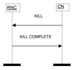
Figure 3: Kill Procedure: Successful Operation
