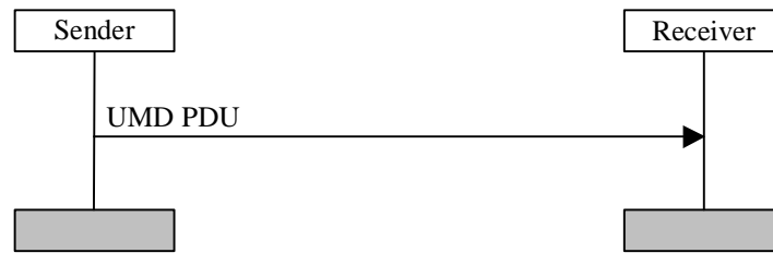
Figure 11.2: Unacknowledged mode data transfer procedure
