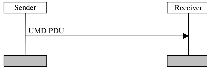
Figure 11.2: Unacknowledged mode data transfer procedure
