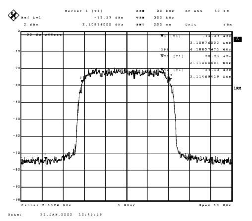
The measurements on the "LLI" interface of the third manufacturer have been more complete, because it was easier to generate channel models and it was possible to disconnect the power amplifier without stopping RF transmission. The results of the measurements for the third supplier are the next:
