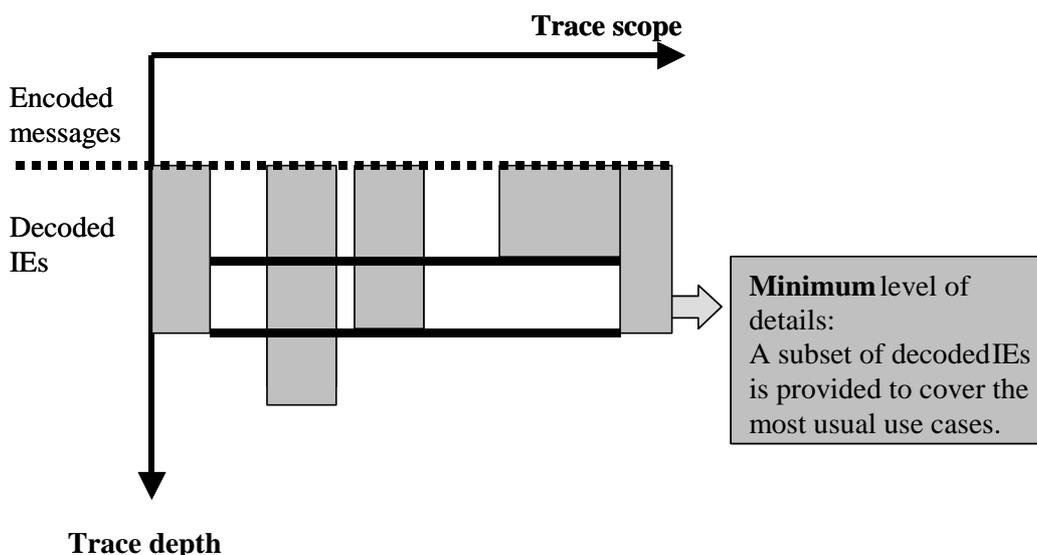
Figure 4: Minimum Level of detail of Trace
