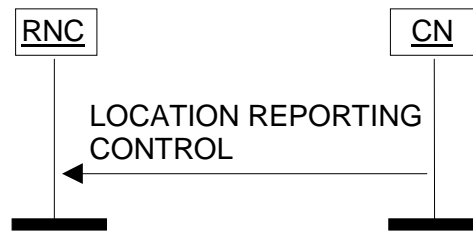
Figure 21: Location Reporting Control procedure. Successful operation.
