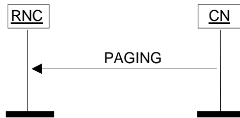
Figure 16: Paging procedure. Successful operation.
