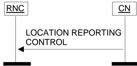
Figure 21: Location Reporting Control procedure. Successful operation.
