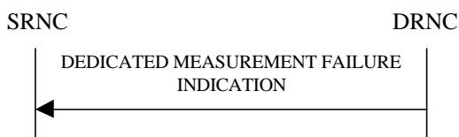
Figure 24: Dedicated Measurement Failure procedure, Successful Operation
