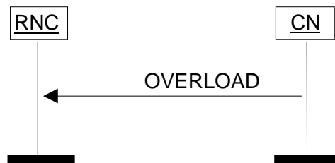
Figure 3: Overload at the CN. Successful operation.
