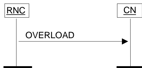
Figure 4: Overload at the UTRAN. Successful operation.
