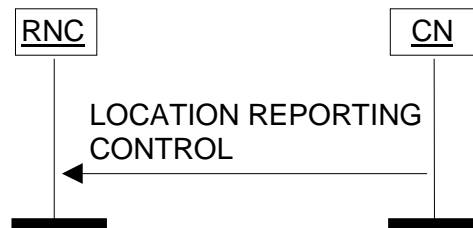
Figure 1: Location Reporting Control procedure. Successful operation.
