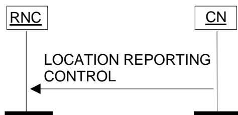
Figure 1: Location Reporting Control procedure. Successful operation.
