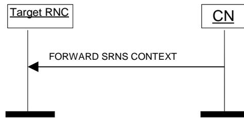
**Figure 2: SRNS Context forwarding to target RNC from CN. Successful operation.**
