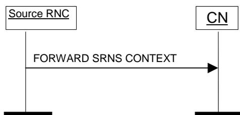
**Figure 1: SRNS Context forwarding from source RNC to CN. Successful operation.**
