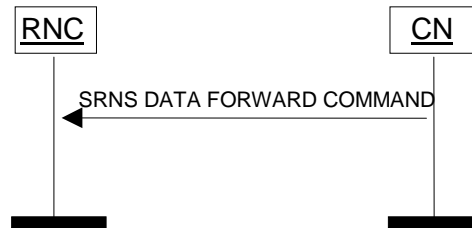
Figure 3: SRNS Data Forwarding Initiation procedure. Successful operation.
