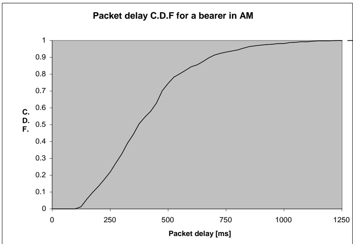
Figure 2 - Simulated packet delay C.D.F. for DCH using RLC AM
