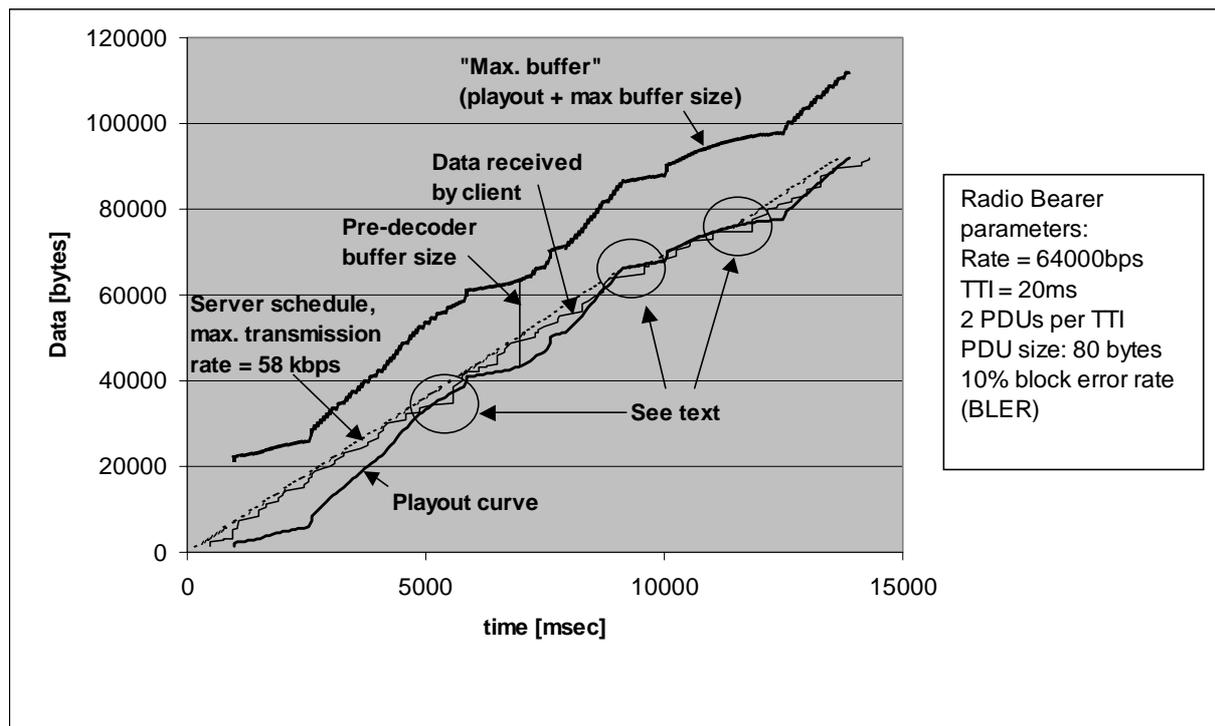
Figure 1 - Impact of the delay jitter introduced by a DCH with RLC AM on streaming playout performance.
