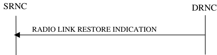
Figure 19: RL Restoration procedure, Successful Operation
