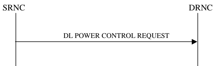
Figure 25: Downlink Power Control procedure, Successful Operation
